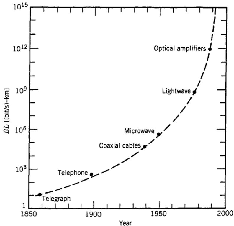
Figure 1.2: Increase in bit rate-distance product  $BL$  during the period 1850-2000.
