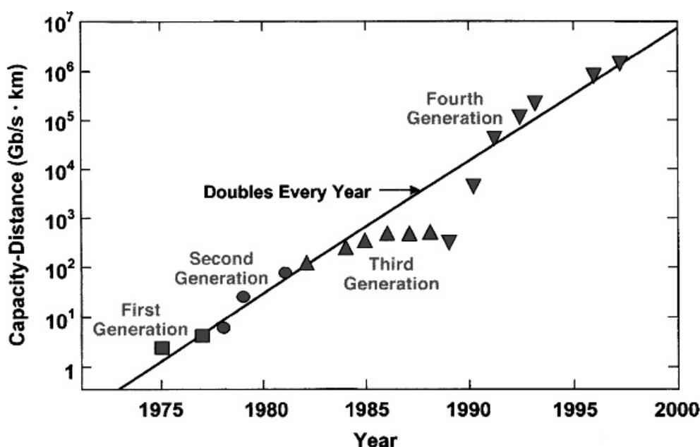
Figure 1.3: Increase in the BL product over the period 1975 to 1980 through several generations of lightwave systems. Different symbols are used for successive generations.
