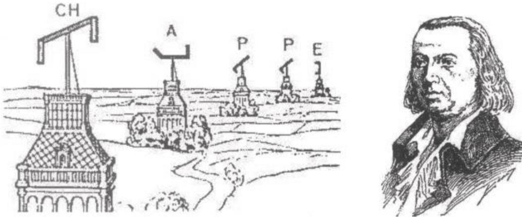
Figure 1.1: Schematic illustration of the optical telegraph and its inventor Claude Chappe.
