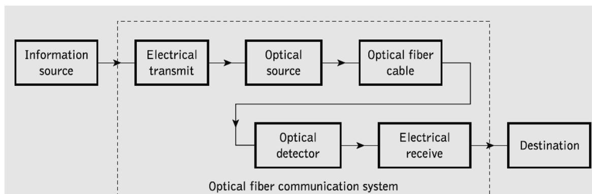
Figure 1.5: Optical fiber communication system.
