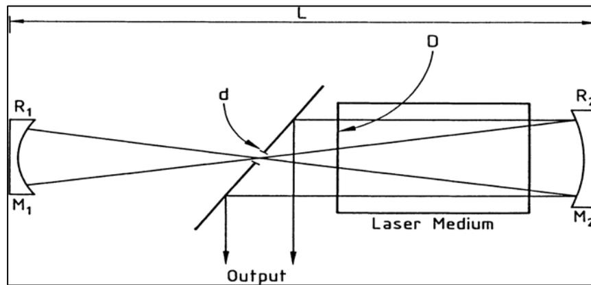
Fig.4 Arrangement of a typical negative-branch unstable resonator
