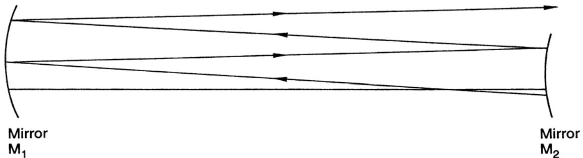
Fig.1. Light ray in an unstable resonator
