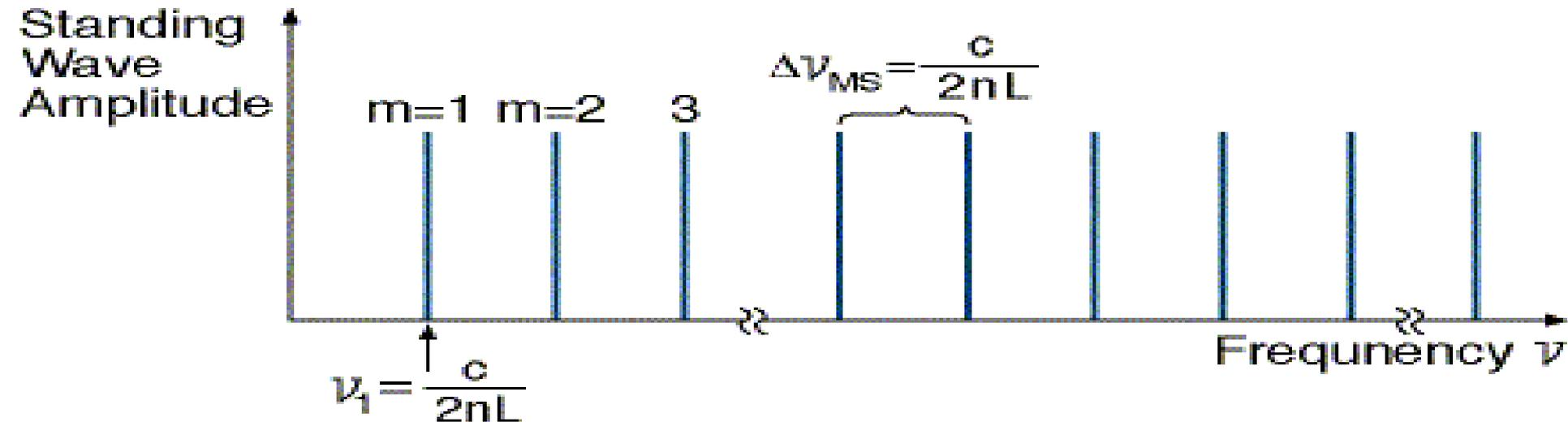
Allowed Longitudinal modes inside a Laser Cavity of length (L) and index of refraction (n).
