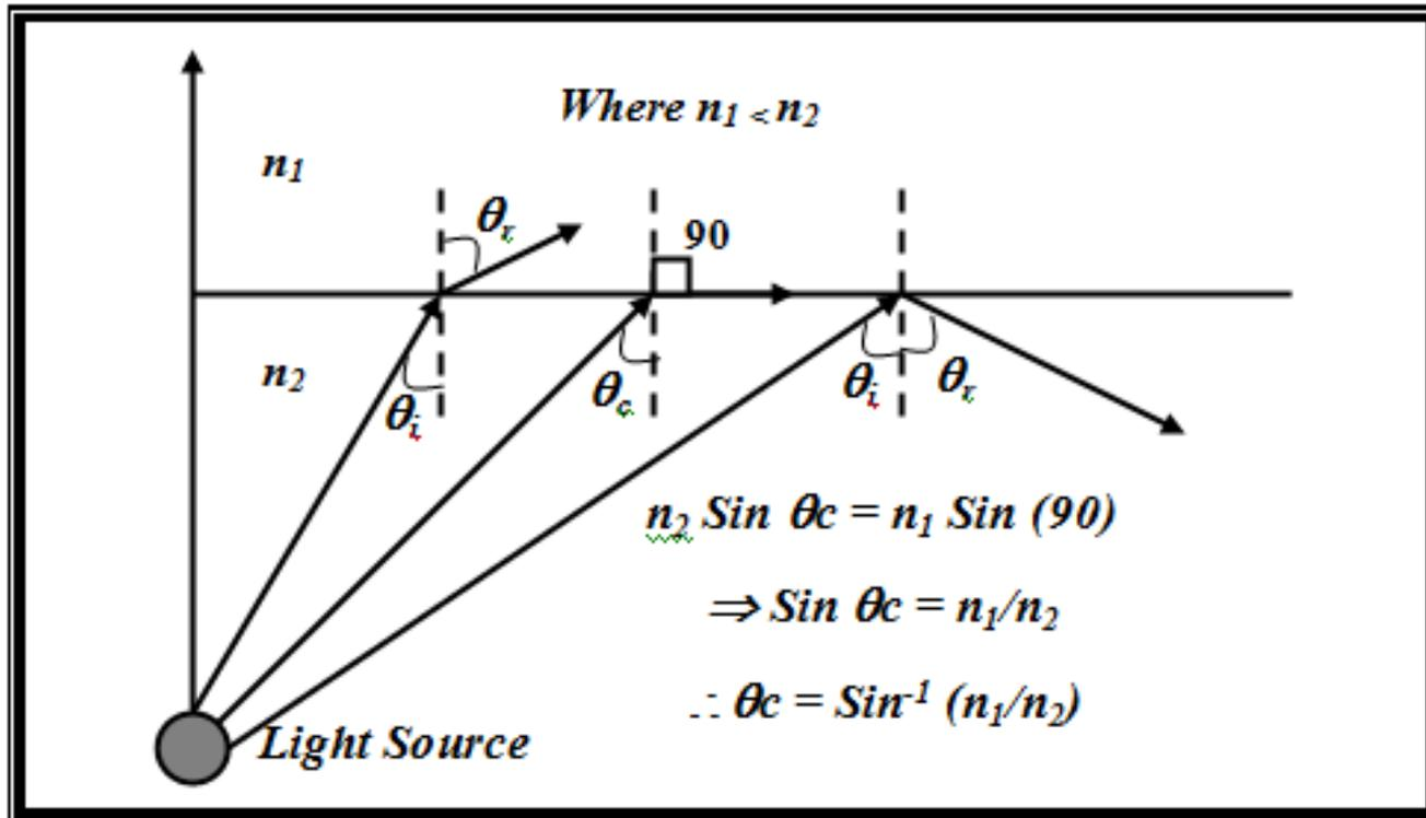
*Figure (1.3) the Total Internal Reflection[5]*
