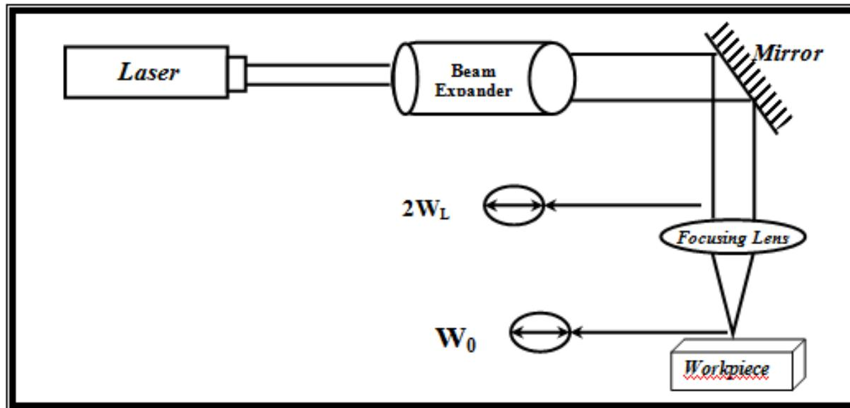
Figure (1.4) Schematic layout of a laser beam delivery[4]
