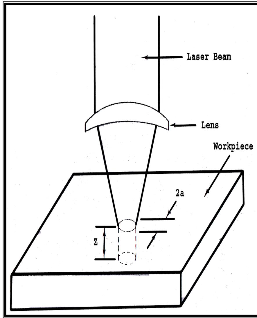
Figure (1.5) Laser beam focused on a workpiece[2]
