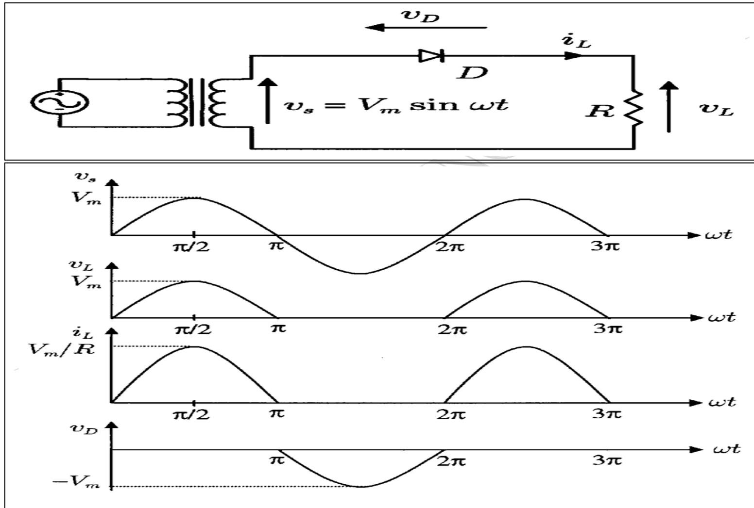
The root-mean-square (rms) value of load voltage  $v_L$  is  $V_L$ , which is defined as:
