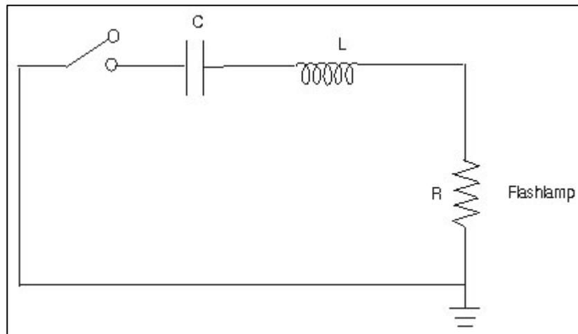
**Fig. 5** RLC discharge circuit
