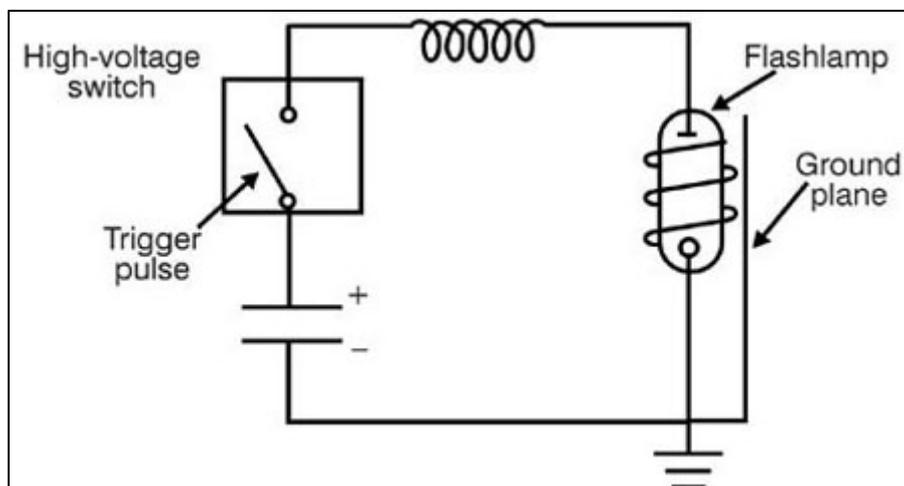
**Fig. 1** Over voltage trigger circuit
