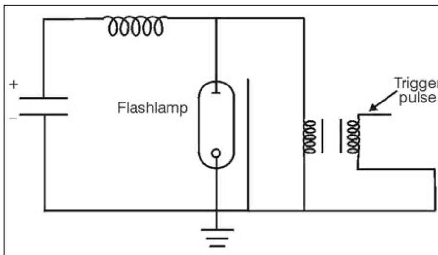
**Fig. 4** Parallel trigger circuit
