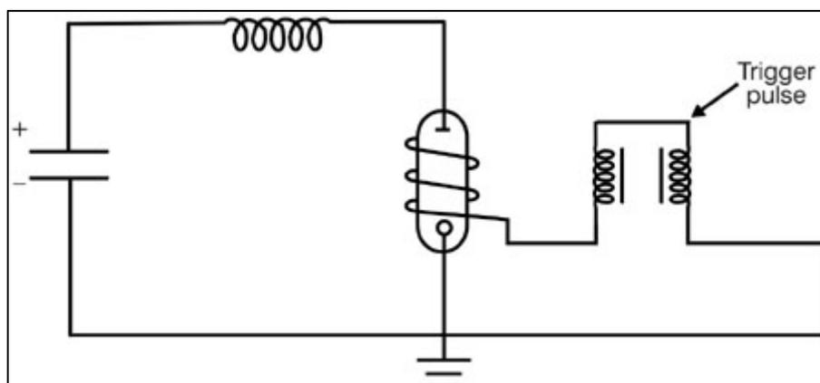
**Fig. 2** External trigger circuit
