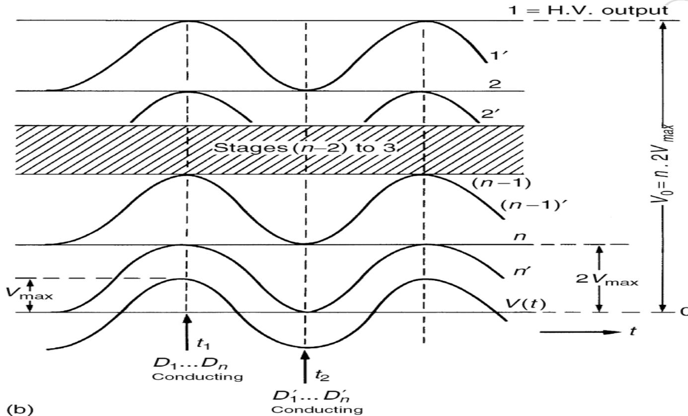
The current through  $D_n$  that charged the capacitor  $C_n$  was not provided by  $D'_n$ , but from  $V(t)$  and  $C'_n$ . We can assume that the voltage across  $C_n$  is not reduced if the potential n' oscillates between zero and  $+2V_{max}$ . If the potential of n', however, is zero, the capacitor  $C'_{n-1}$  is also charged to the
