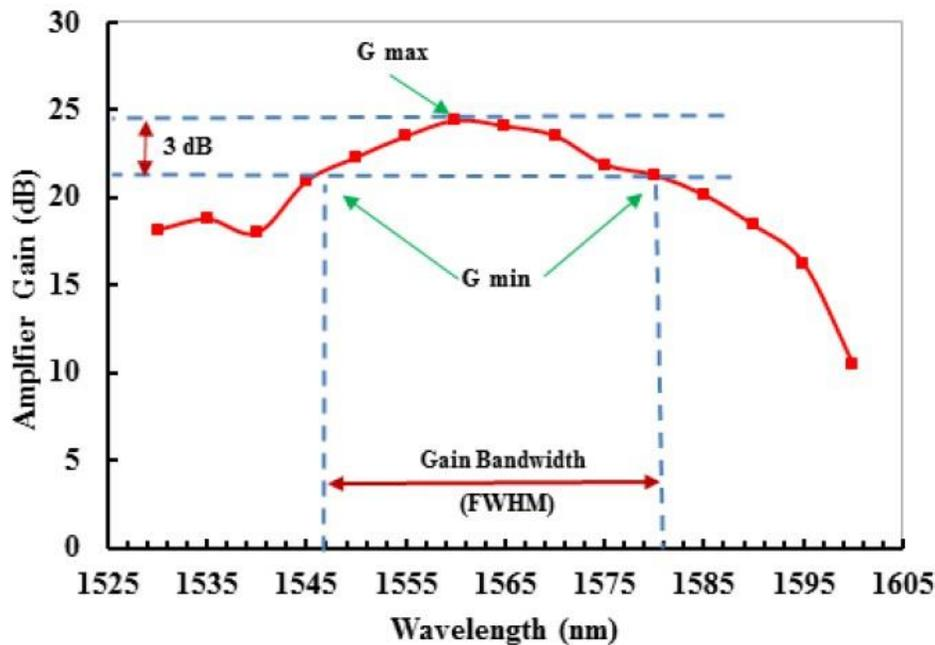
Figure 4.2: Gain parameters used to evaluate the amplifier gain.
