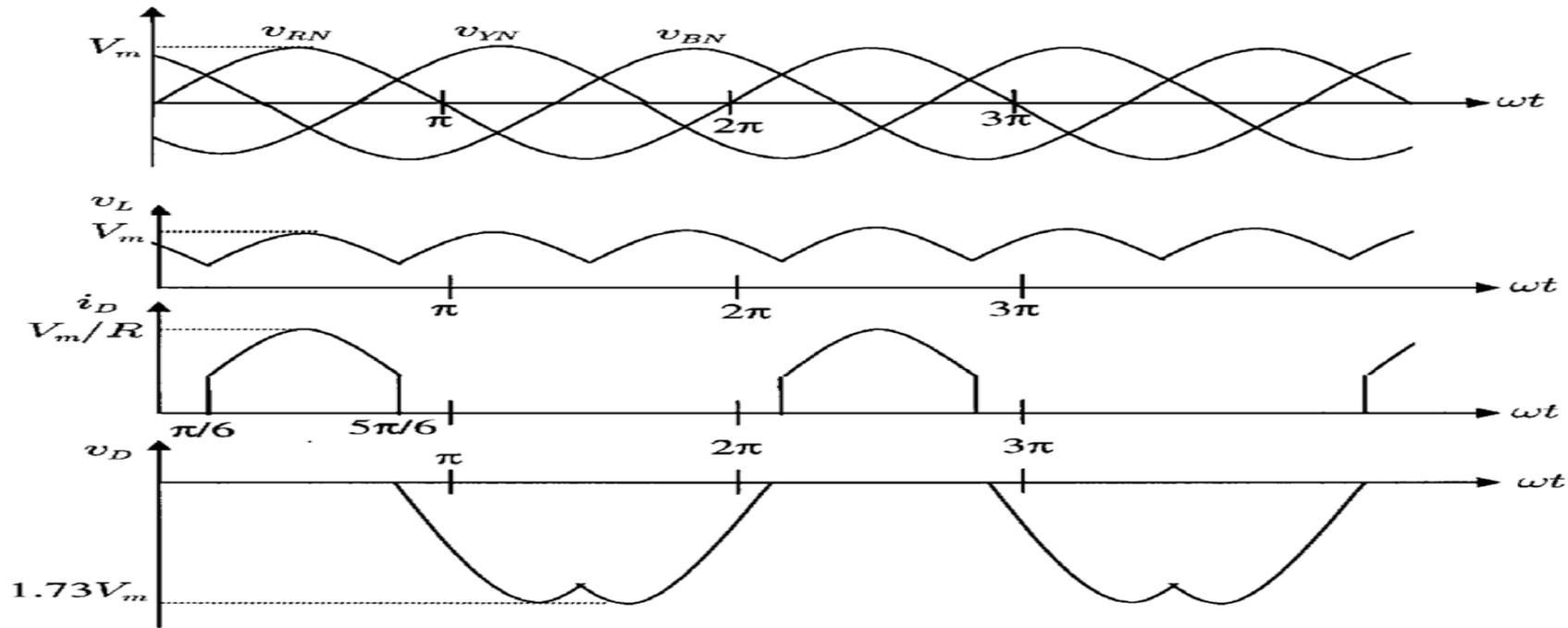
→ It is clear that, unlike the single-phase rectifier circuit, the conduction angle of each diode is  $2\pi/3$ , instead of  $\pi$ .
