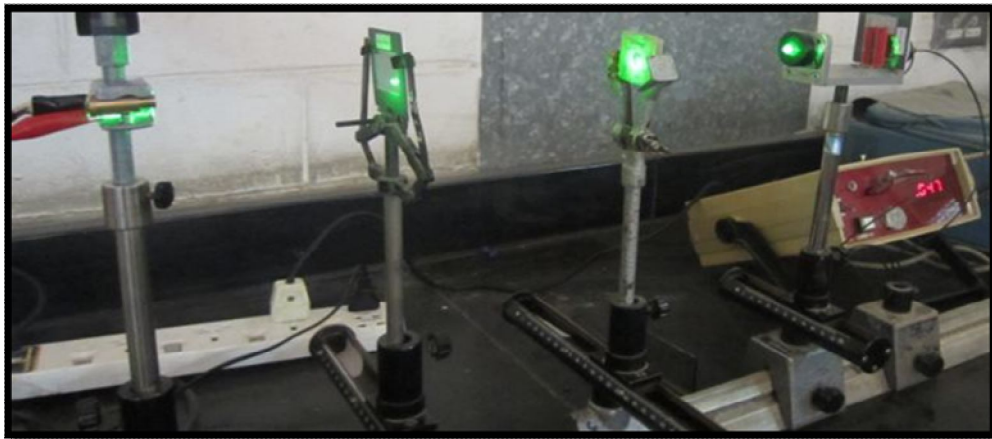
Figure 1 shows Experimental arrangement for bulk sample measurement using polarization technique to measure Hb concentration
