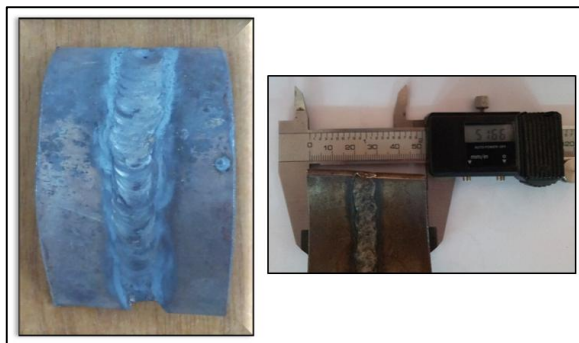
Figure 1: Specimen after welding
